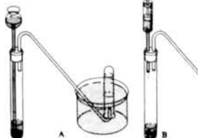
2.33 Collecting hydrogen gas
