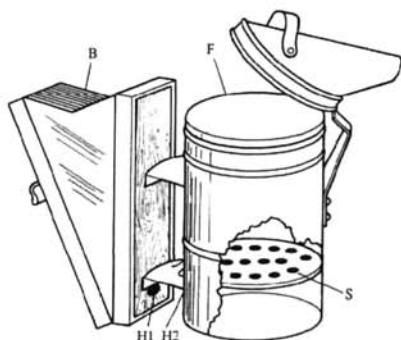
FIG. 68. Diagram of a smoker. B – Bellows; H1 and H2 – Air holes; F – Fire box; S – Shelf for fuel. This is the most vital piece of equipment for opening hives and removing frames that have been stuck in with propolis.
