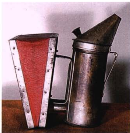
FIG. 67. The Smoker. This is an important piece of equipment as it helps to keep the bees calm during hive operations.
