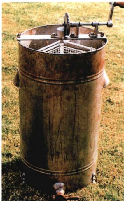
FIG. 70. Honey extractor. This provides a mechanical method for removing honey from combs. In this device two, three or four combs are placed in the drum with their surfaces towards the walls. When the handle is turned they spin and the honey from the uncapped combs is thrown onto the walls of the drum. It runs to the bottom and then can be poured out using the tap. It usually stands on a bench so that a bucket can be placed under the tap.
