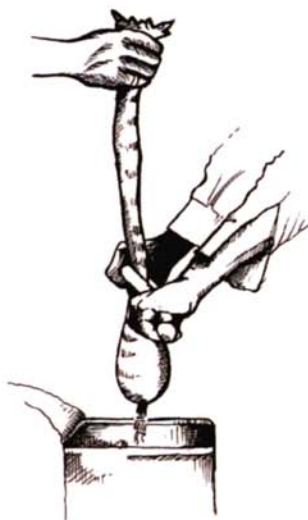
FIG. 79. Straining wax. Beeswax, which has been melted in water, is scooped up and put through a bag of coarse fibres that can be squeezed using two parallel sticks as well as wringing the bag with the hands.
