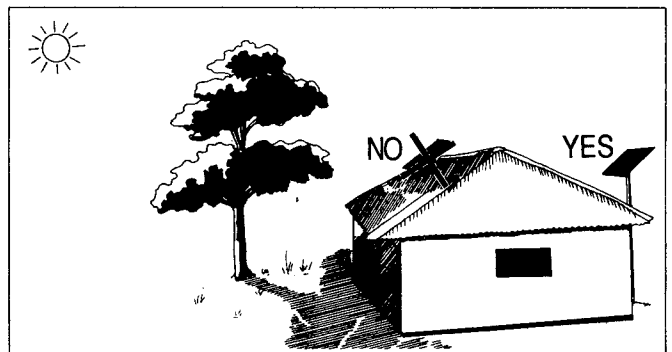
Figure 11.4 Module site. Do not place module where it might be shaded by trees or obstructions.
